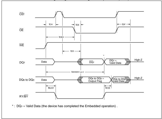
• AC Waveforms for Data Polling during Embedded Algorithm Operations (Flash)
