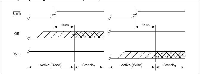
Note : Both t<sub>CHOX</sub> and t<sub>CHWX</sub> define the earliest entry timing for Standby mode. If either of timing is not satisfied, it takes t<sub>RC</sub> (Min) period from either last address transition of A<sub>0</sub> and A<sub>1</sub>, or CE1r Low to High transition.
