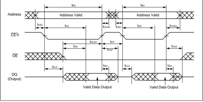
Note : CE2r and  $\overline{\text{WE}}$  must be High for entire read cycle.
