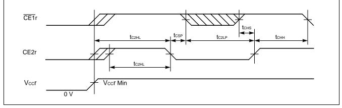
\* : The tc2LH specifies from CE2r Low to High transition after Vccr reaches specified minimum level. CE1r must be brought to High prior to or together with CE2r Low to High transition.
