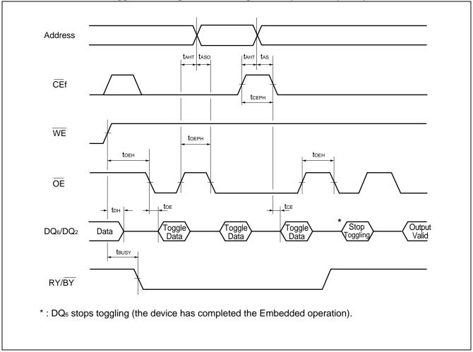
• AC Waveforms for Toggle Bit during Embedded Algorithm Operations (Flash)
